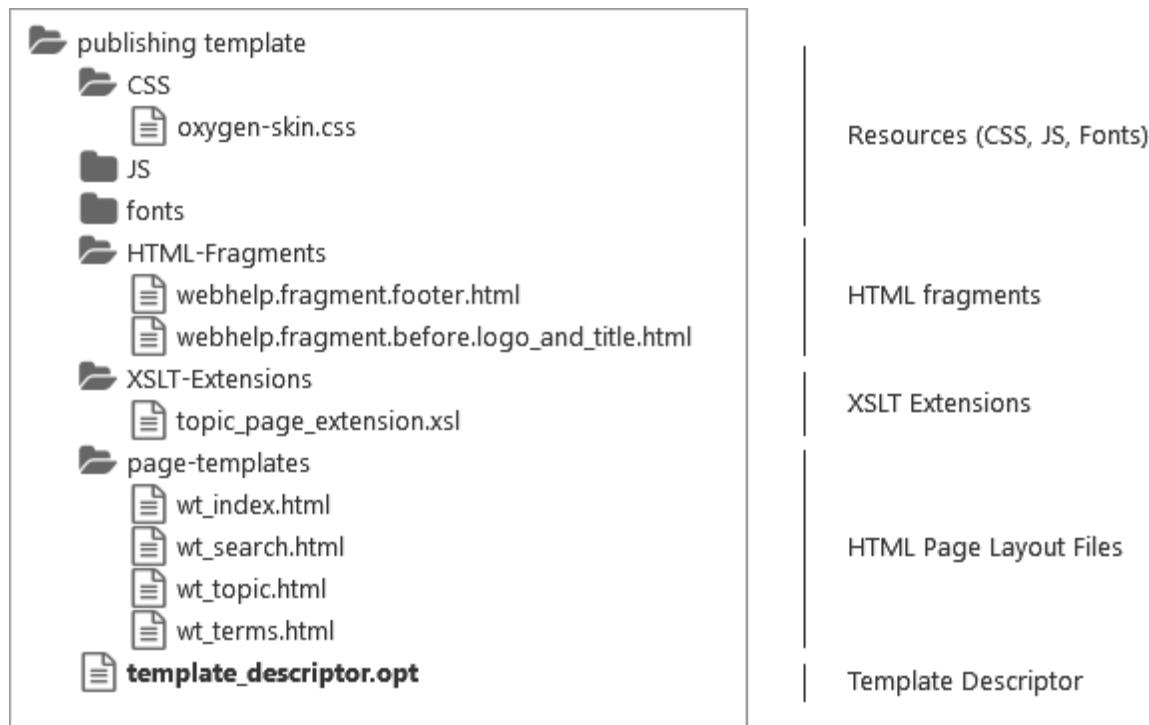
**Figure 2. Oxygen Publishing Template Package (PDF)**
